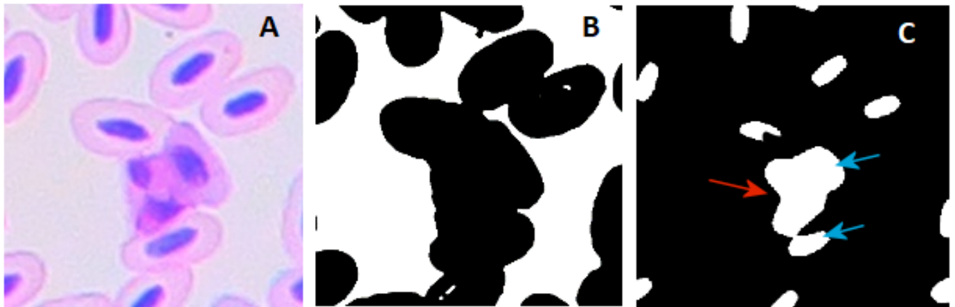
Figure 6. Example of a cell identification error where a heterophil is closely pressed against a RBC. The cell outline detection has grouped the touching cells together (B). Typically, the nucleus identification process (C) separates the cells, but here it has merged together the nuclei of the heterophil (red arrow) and two red blood cells (blue arrows).
