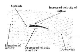
The more the wing is tilted against the airflow, that is, the **greater the angle of attack** of the airflow against the wing, the greater the curvature of the airflow over the top surface, the greater the deflection downwards underneath, and the greater the lift.
